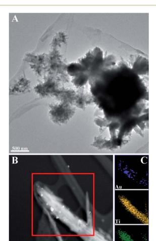
Fig. 3 TEM images of Au NCs deposited  $TiO_2$ -NRs(150): (A) morphology of  $CNC/TiO_2$ -NRs(150)/Au NCs; (B) HAADF STEM micrograph of  $TiO_2$ -NRs(150)/Au NCs and corresponding (C) EDS mapping of Au, Ti and O.
