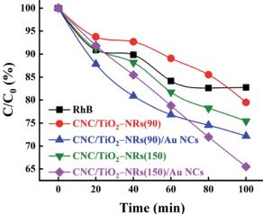
Fig. 5 Photodegradation of RhB (8 ppm in 50 mL of aqueous solution) under simulated sunlight on different photocatalysts (200 mg, powder) supported by  $H_2O_2$ . The solution was illuminated with 100 mW cm<sup>-2</sup> AM 1.5G illumination (1 sun).
