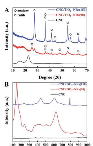
Fig. 2 (A) XRD patterns of CNC, CNC/ $TiO_2$ -NRs(90) and CNC/ $TiO_2$ -NRs(150) and (B) Raman patterns of CNC, CNC/ $TiO_2$ -NRs(90) and CMC/ $TiO_2$ -NRs(150).
