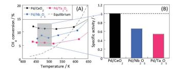
Fig. 1 (A) Temperature dependence of catalytic MSR activity in the electric field and (B) specific activity at 473 K. Reaction conditions: preset temperature, 323-773 K (ER); catalyst weight, 100 mg; flow,  $CH_4: H_2O: Ar = 1: 2: 7$ , total 100 SCCM; current, 9 mA.
