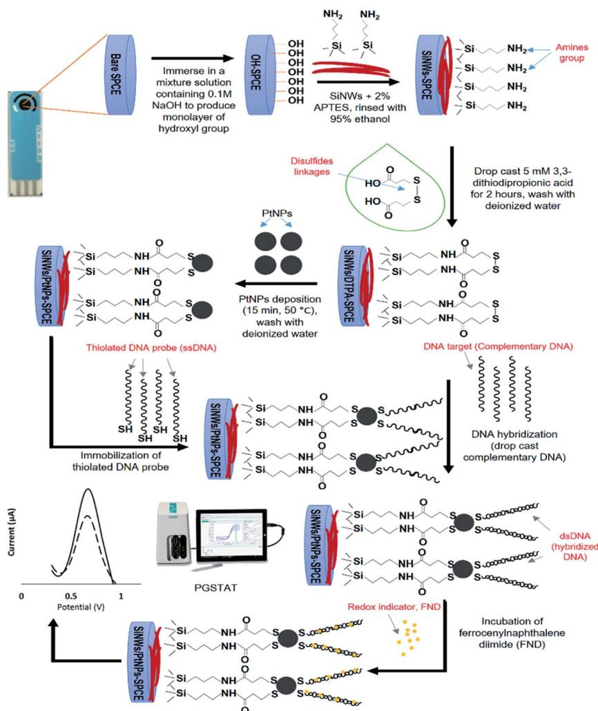
Fig. 2 Schematic illustration of the fabrication and DNA hybridization process of SiNWs/PtNPs modified SPCE for electrochemical biosensor.
