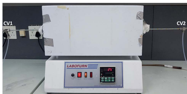
Fig. 1 Image of reactor and furnace setup, under argon atmosphere with a feed of 2 bar at room temperature, when heated to 350 °C. The manual control valves (CV1 and CV2) are open during purging (~1 h) and closed after initial purge. The quartz wool in the reactor outlet is to contain the precursors in the reactor and a beaker filled with water on the exit flow is placed while flowing Ar to monitor the gas flow and prevent air from entering the reactor.
