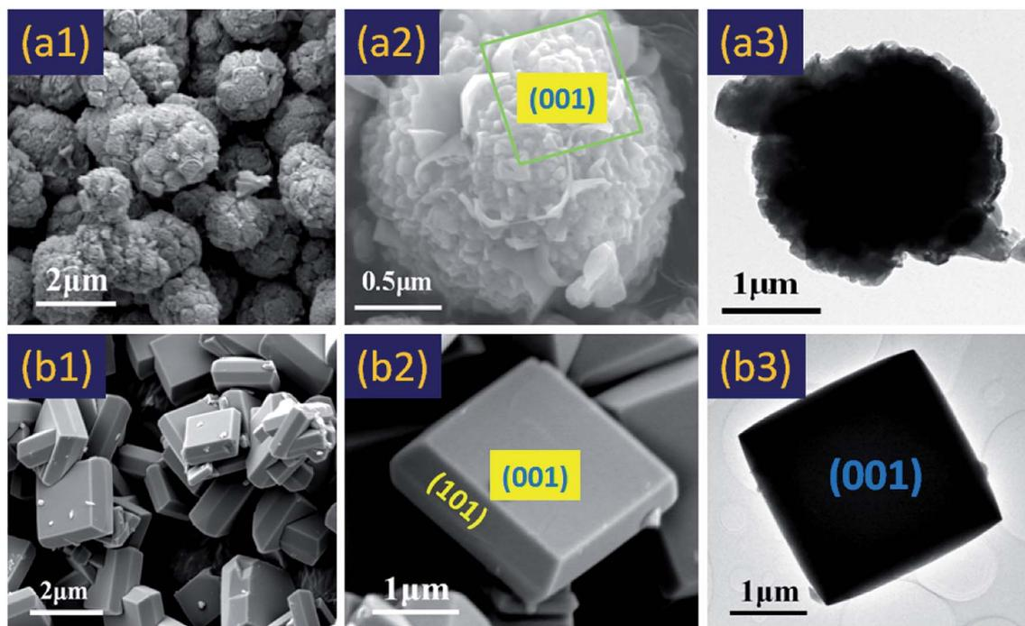
Fig. 1 Microstructure and morphology of anatase TiO<sub>2</sub> crystals. (a1), (a2) and (a3), SEM and TEM images of typical spherical TiO<sub>2</sub> polycrystalline particles (without HF). (b1), (b2) and (b3), SEM and TEM images of typical anatase TiO<sub>2</sub> single crystals (with HF).
