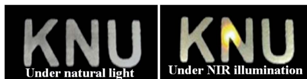
Fig. 9 KNU Log mark prepared using the optimized \text{TiO}_2:\text{Er}^{3+}/\text{Yb}^{3+} spherical particles under natural light (left) and when irradiating with a portable 980 nm IR lamp (right).
