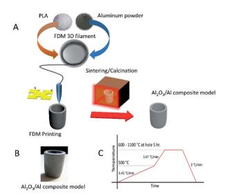
Fig. 1 (A) Schematic of the fabrication of the  $Al_2O_3/Al$  composite refractory. (B) The  $Al_2O_3/Al$  composite refractory after sintering and calcination. (C) Temperature profile during the sintering and calcination process.
