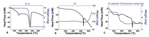
Fig. 2 (A), (B) and (C) DSC and TGA of PLA, Al, and the as-printed Al/polymer-composite, respectively. The phase transformation of the as-printed Al/polymer-composite was the same as those of PLA and Al in combination.
