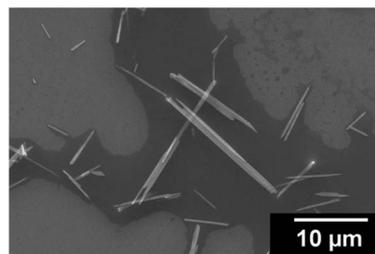
Fig. 2 SEM image of MoO<sub>3</sub> crystals.
