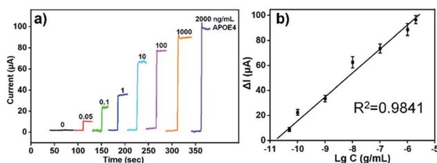
Fig. 4 (a) Amperometric *i-t* results of the APOE4 immunosensor for reduction of H<sub>2</sub>O<sub>2</sub> (2 mM) under constant stirring when detecting different concentrations of human APOE4 protein range from 0.05 ng mL<sup>-1</sup> to 2000 ng mL<sup>-1</sup>. (b) Calibration curve of the designed immunosensor for the detection of APOE4. The equation:  $\Delta I = 18.191 \lg C + 200.78$ ,  $R^2 = 0.9841$ . Error bar = relative standard deviation ( $n = 3$ ).
