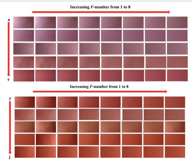
Fig. 2 The images recorded for the samples of the test set: (a) 1, (b) 2.5, (c) 15, (d) 50, (e) 90, (f) 150, (q) 300, (h) 500, (i) 700 and (j) 900 ppm nitrite.
