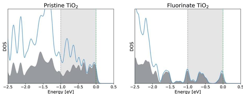
Fig. 2 The density of states computed for the pristine TiO<sub>2</sub> (left) and the fluorinated TiO<sub>2</sub> (right) is shown in blue with the contribution from the interfaces shown in grey. In each case, the Fermi level (green dashed line) was shifted to 0 eV. The 1 eV region of the density of states used to compute the two-dimensional DOS is highlighted between the two dashed lines.
