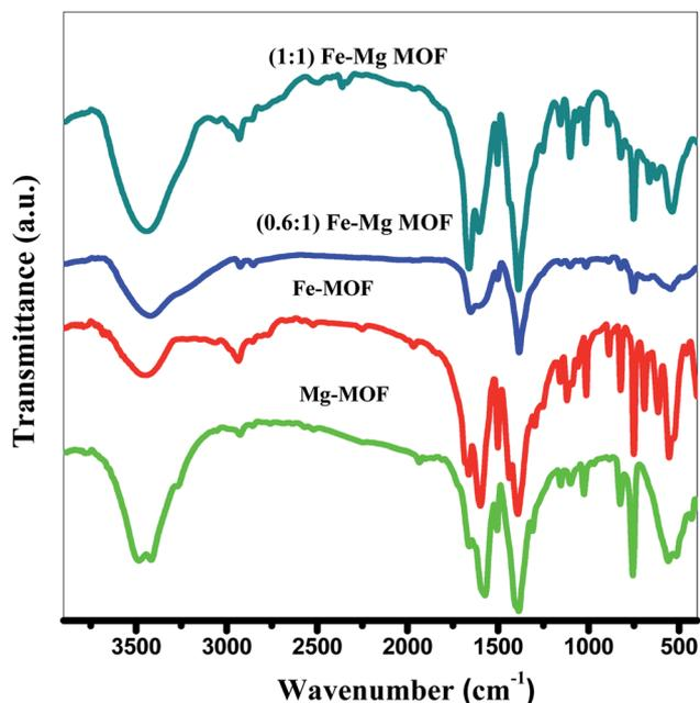
Fig. 1 FTIR spectra of the prepared MOFs.
