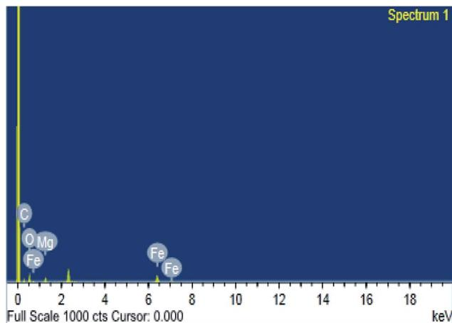
Fig. 4 EDS image of (0.6 : 1) Fe-Mg MOF.
