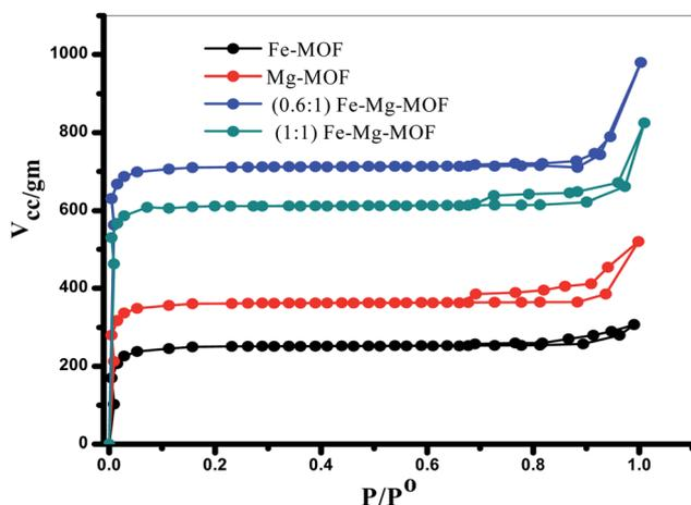
Fig. 5  $N_2$  adsorption-desorption isotherms of the prepared MOFs.
