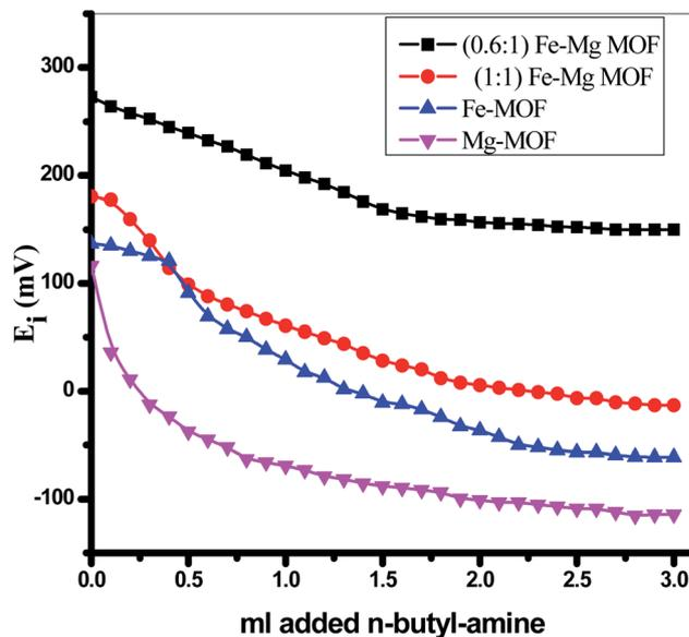
Fig. 6 Nonaqueous potentiometric titration for the prepared MOFs.
