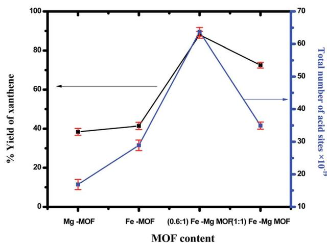
Fig. 7 Effect of the total number of acid sites of the prepared MOF on synthesis of 14-aryl-14-*H*-dibenzo[*a,j*]xanthenes. The error bars represent the standard error.
