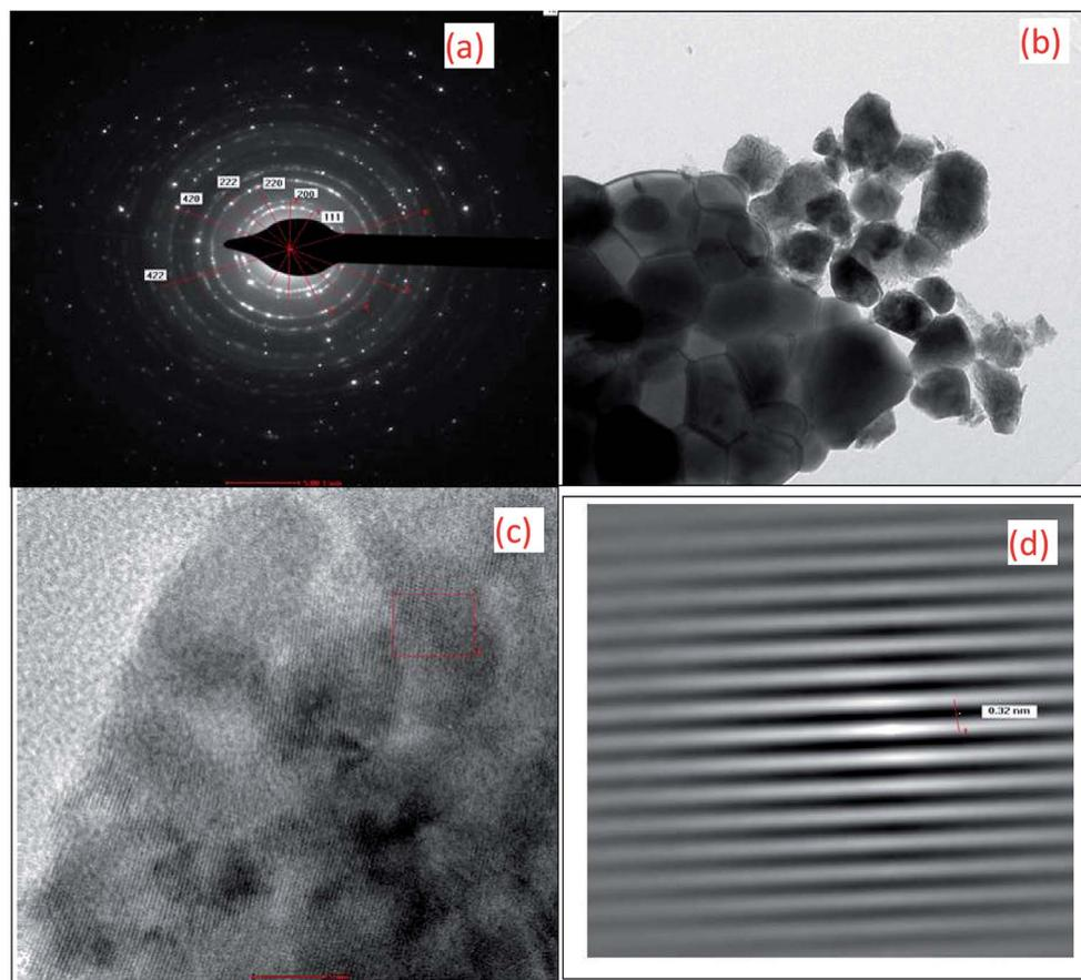
**Fig. 3** TEM images of 10GDC sintered at 1200 °C for 4 h in the microwave furnace: (a) SAED pattern, (b) TEM image, (c) HRTEM image (d) the enlarged view of the marked portion of (c), which was used for measuring the *d*-spacing value.
