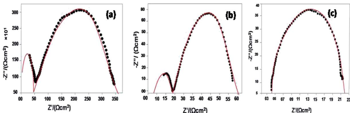
Fig. 7 EIS spectra of 10GDCs sintered at 1200 °C in presence of O<sub>2</sub> = 1 atm for the operating temperatures of (a) 600 °C, (b) 700 °C, and (c) 800 °C.
