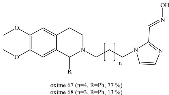
Fig. 24 Chemical structure of oximes developed by Wei *et al.* (2014).<sup>81</sup>
