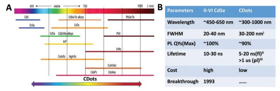
Fig. 4 PL tuning range (A) and comparison of optical properties (B) of TQDs vs. CDots. Reproduced with permission from ref. 29 and 103, Copyright 2016 and 2018, American Chemical Society (FWHM of 30 nm was only reported in ref. 40; "fl: fluorescence; "pl: phosphorescence)
