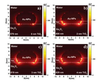
Fig. 4 Near-field distributions of Au-NPs/ $Ga_2O_3$  modified with (a) 0, (b) 2, (c) 3, and (d) 4 nm  $TiO_2$  layers, which was calculated by an FDTD simulation.
