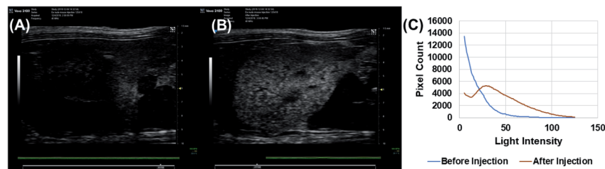
Fig. 9 Ultrasound images of mouse kidney (A) before and (B) after injection of echogenic exosomes ( 100 \mu\text{l} of 58 \text{ mg mL}^{-1} ) into the tail vein of NSG mouse using Vevo 3100 Imaging System and 40 MHz transducer head (at 100% power, 70 fps frame rate, 25 dB gain, depth 10 mm and width 18 mm, 70 dB dynamic range, brightness 50 and contrast 50 for both images). (C) Pixel count differences of light intensity between echogenic exosomes before (blue) and after (red) tail vein injection. Pixel count was normalized by the area for the graph.
