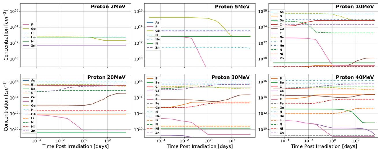
Fig. 5 Total concentrations of impurity elements introduced in Ga<sub>2</sub>O<sub>3</sub> as a function of time following quasi-monoenergetic 2, 5, 10, 20, 30, and 40 MeV proton irradiation. Substantial dopants of note include Ge, N, and Zn for most proton energies ( $E_p$ ), with the inclusion of C for  $E_p \geq 10$  MeV, Cu and Ni for  $E_p \geq 20$  MeV, B for  $E_p \geq 30$  MeV, and Li for  $E_p \geq 40$  MeV. All results are shown in tabular format in the ESI.†
