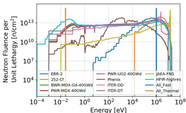
**Fig. 1** Incident neutron spectra, each of which is used as a source for transmutation quantification. More detail concerning these spectra is included in Table 1. For all neutron spectra shown here, the total fluence of  $3.6 \times 10^{17}$  neutrons per  $\text{cm}^2$  is employed (1 hour irradiation in a typical light water reactor of total  $10^{14}$  neutrons per  $\text{cm}^2$  per s scalar flux).
