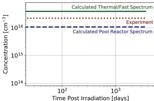
Fig. 2 Comparison between experimentally observed<sup>26</sup> and computed Ge concentration resulting from GaN neutron irradiation with thermal and fast neutron fluence of  $1.5 \times 10^{17}$  neutrons per  $\text{cm}^2$  for pure thermal and pure fast neutron spectra and for a similar thermal pool-type light water reactor as was used for experimental irradiation. Concentrations are shown starting at 3 weeks post-irradiation, as this was when the experiment was performed.
