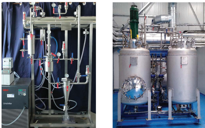
Fig. 4 Lab and industrial scale liquefied gas extraction systems from CELSIUS-France.
