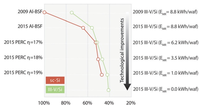
Fig. 6 Change in climate change impact scores as a result of technological improvements. 2009: Reference data (2009) for silicon, module and BOS supply chains from ecoinvent v3.4; 2015: Updated IEA PVPS data (2015) for silicon, module and BOS supply chains; \eta : module efficiency; E_{MR} : Energy consumption for a single MOVPE run of 31 wafers; waf: calculations based on a 156 \times 156 \text{ mm}^2 wafer.
