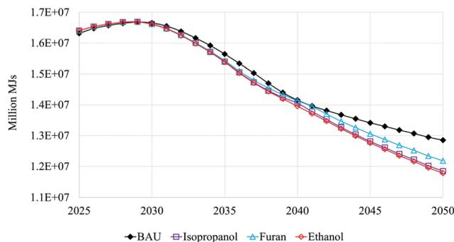
Fig. 5 Petroleum fuel consumption, in million Btus, of isopropanol, furan, and ethanol cases, in comparison to the BAU case.
