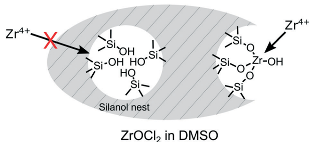
Fig. 20 Schematic representation of Zr grafting to generate “open” Zr(IV) sites by treatment of dealuminated \beta zeolite with \text{ZrOCl}_2 in DMSO. Reproduced from ref. 217. Copyright 2017, with permission from John Wiley & Sons, Inc.
