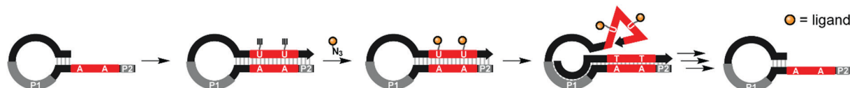
Fig. 5 SELMA (selection of modified aptamers) process: a library of hairpins is extended by polymerase which incorporates alkyne-modified uridines. Azide-modified ligands are conjugated through Cu-mediated click chemistry. Extension from primer site P1 ejects the ligand-decorated strand from the hairpin, allowing it to fold into a three-dimensional shape, which is screened against a target compound. Through multiple subsequent steps the starting hairpin can be regenerated for further selection rounds (ref. 21).
