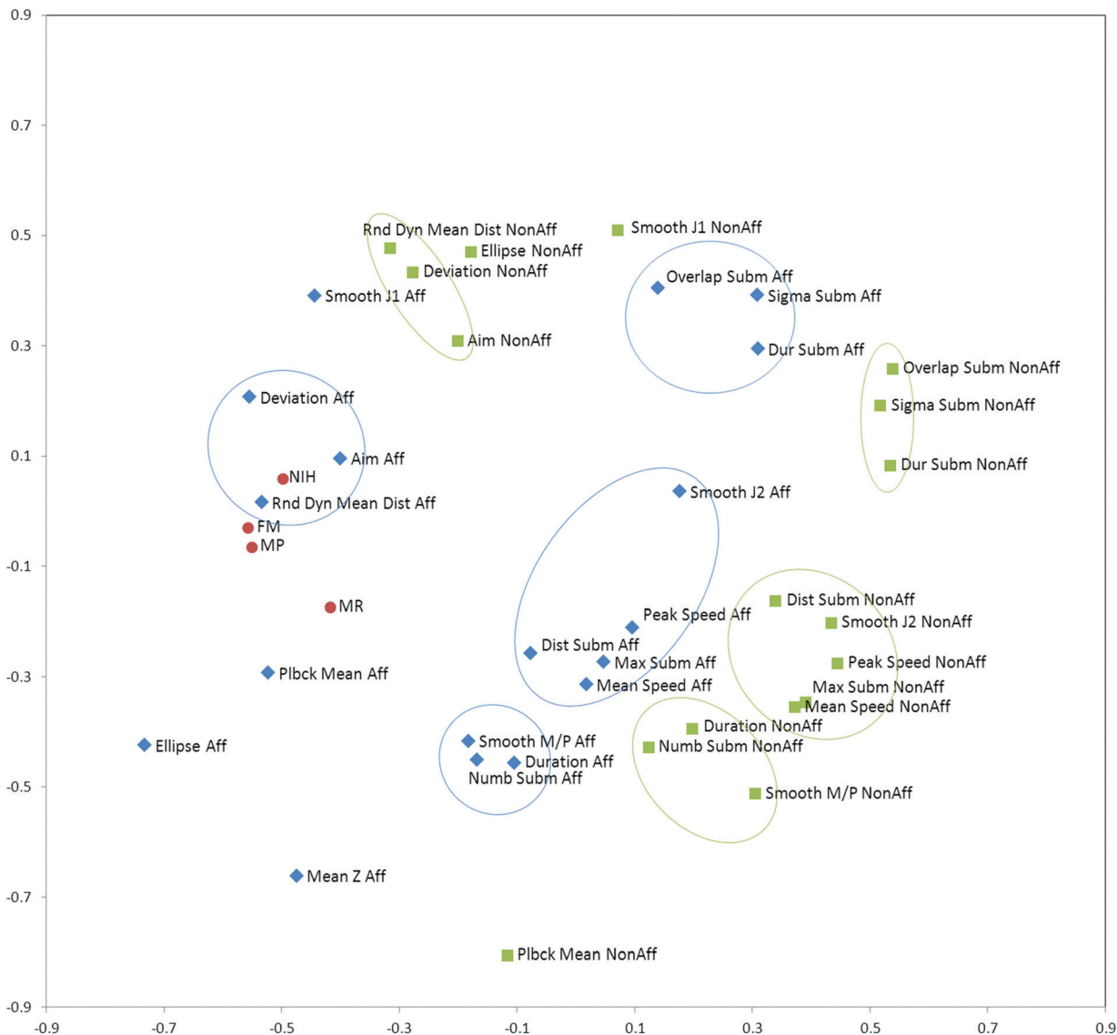
Fig. 12 SPE map of the correlation distances of the clinical and robotic parameters for the completers cohort. The map was derived by computing the pairwise Pearson correlation coefficients ( R ) for all pairs of features, converting them to correlation distances ( 1 - \text{abs}(R) ), and embedding the resulting matrix into 2 dimensions in such a way that the distances of the points on the map approximate as closely as possible the correlation distances of the respective features. The clinical parameters are highlighted in red, the robotic parameters on the affected side in blue, and the robotic parameters on the unaffected side in green. The map also shows distinct clusters of correlated variables which are preserved on both the affected and unaffected sides (outlined by green and blue ellipses, respectively).
