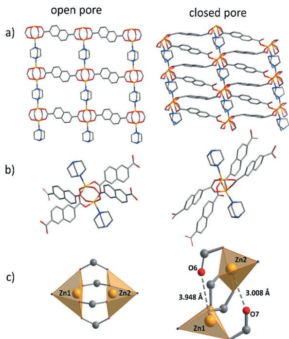
**Fig. 2** Crystal structure of: a) **1<sub>op</sub>** and **1<sub>cp</sub>** along *b* direction; b) the coordination environment of the Zn paddle wheel unit in: **1<sub>op</sub>** and **1<sub>cp</sub>**; c) view on coordination polyhedron of **1<sub>op</sub>** and **1<sub>cp</sub>**. C – in grey, O – in red, N – in blue, Zn – in yellow. Hydrogen atoms are omitted for clarity.
