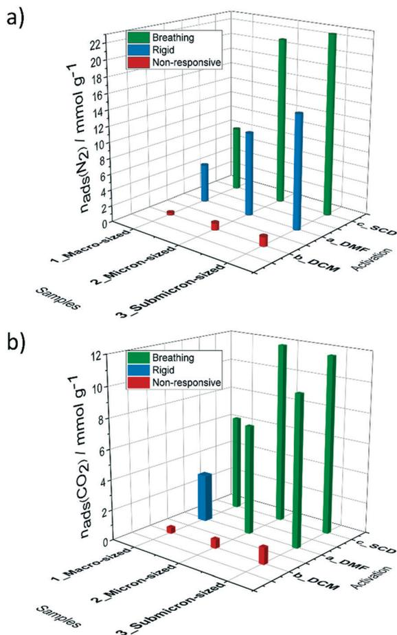
Fig. 8 Comparison of a) nitrogen (77 K) and b) carbon dioxide (195 K) uptake and structural response depending on particle size and activation strategy.
