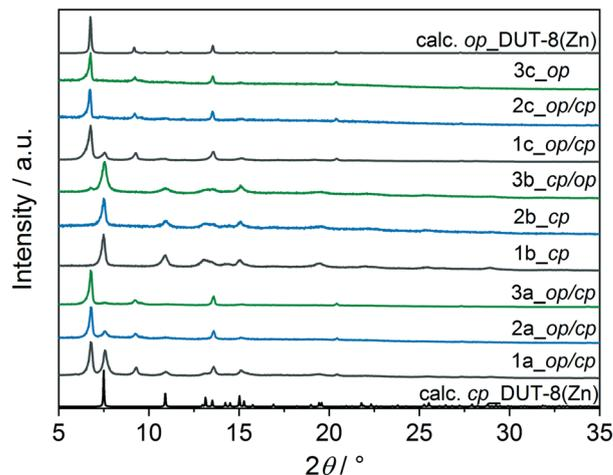
Fig. 4 PXRD patterns of **1**-macro-, **2**-micron-, **3**-submicron-sized particles of DUT-8(Zn) after different solvent removal procedures applied: (a) indicates desolvation from DMF in vacuum at 423 K, (b) indicates desolvation from DCM in vacuum at 423 K and (c) indicates desolvation using SCD. The calculated pattern of the op and cp phases DUT-8(Zn) are given for comparison.
