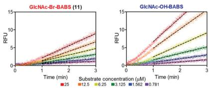
Fig. 11 BABS probes 41 and 44 are turned over by hOGA. Evolution of fluorescence (RFU) for different concentrations of 41 and 44 in the presence of hOGA. Dotted lines represent the linear rates reached at steady state, adapted with permission from ref. 58
