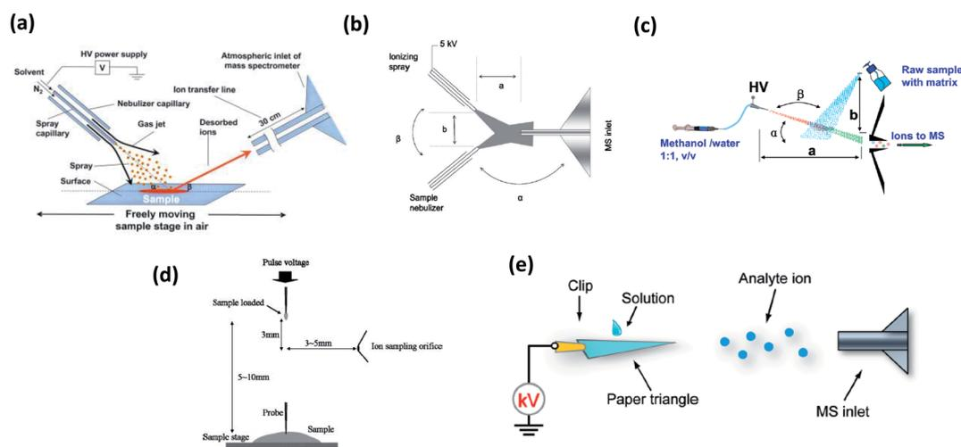
**Fig. 2** Schematic representations of (a) DESI (ref. 10); (b) EESI (ref. 45); (c) nanoEESI (ref. 49); (d) PESI (ref. 74); (e) PS-MS (ref. 59). For details, see text. Adapted with permission from the publishers (Wiley, Royal Society of Chemistry, ACS and AAAS).
