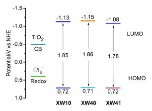
Fig. 3 Schematic energy-level diagram of XW10,33 XW40 and XW41.
