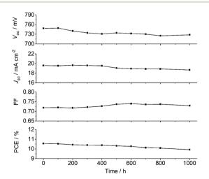
Fig. 8 Variation of the photovoltaic parameters ( $V_{oc}$ ,  $J_{sc}$ , FF, and PCE) with aging time for the DSSC device based on XW40/CDCA + Z1 measured under AM 1.5 illumination (100 mW  $cm^{-2}$ ) at 60  $^{\circ}$ C over 1000 h.
