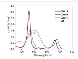
Fig. 2 Absorption spectra of the porphyrin dyes and the cosensitizer Z1 in THF.
