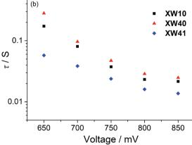
Fig. 7 Plots of (a)  $C_{ij}$  and (b)  $\tau$  versus bias voltages of DSSCs based on XW10, XW40, and XW41.
