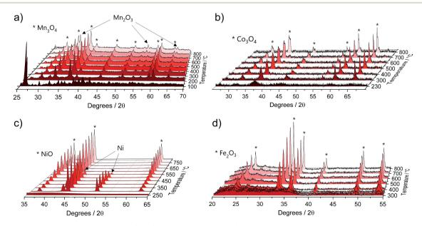
Fig. 2 Selected in situ XRD spectra of the pure  $M(acac)_x$  (M = Mn, Co, Ni and Fe) precursors acquired in air within a temperature range of 25 °C to 800 °C and heating rate of 5 °C min<sup>-1</sup> for (a)  $Mn(acac)_2$ , (b)  $Co(acac)_3$ , (c)  $Ni(acac)_2$  and (d)  $Fe(acac)_3$ . Full data sets can be found in Fig. S2.†
