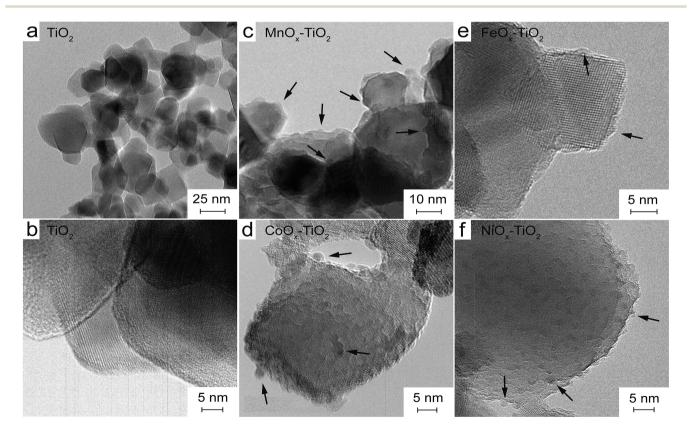
Fig. 4 TEM pictures of the  $TiO_2$  NPs (a and b) as well as  $MnO_x$ – $TiO_2$  (c),  $CoO_x$ – $TiO_2$  (d),  $FeO_x$ – $TiO_2$  (e) and  $NiO_x$ – $TiO_2$  (f) composites prepared at 350 °C. Arrows indicate examples of clearly visible  $MO_x$  species.
