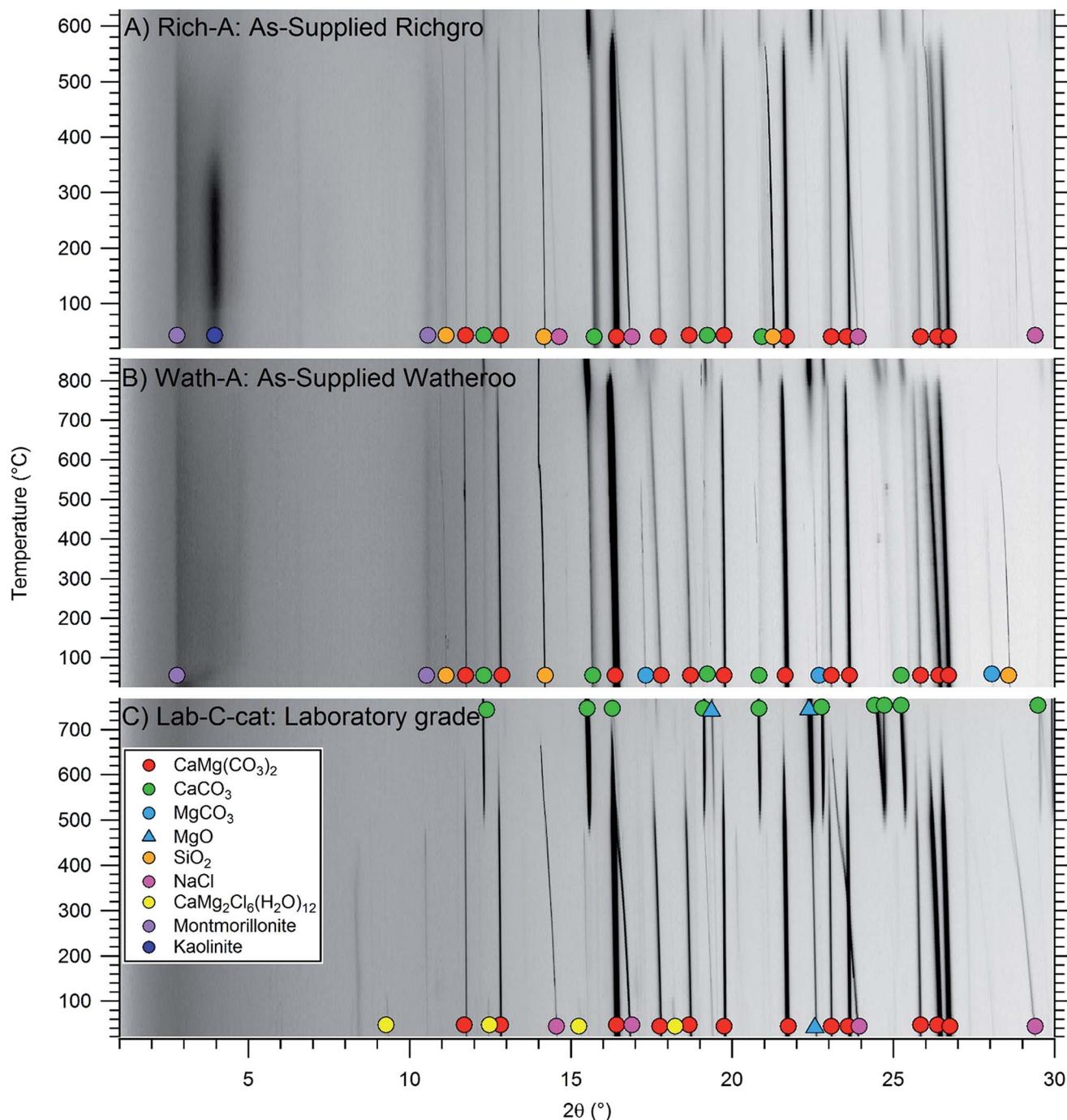
Fig. 2 *In situ* powder X-ray diffraction of (A) Richgro, (B) Watheroo and (C) Laboratory grade dolomite samples heated at  $6\text{ °C min}^{-1}$  under 1 bar Ar. ( $\lambda = 0.8263076\text{ \AA}$ ). The same primary end products are formed in all three samples under these conditions of temperature and time.
