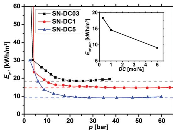
Fig. 13 The specific energy  $E_{m^3}$ , calculated by eqn (12), is plotted as a function of the applied pressure for 0.3, 1 and 5 mol% crosslinked PSA hydrogels. The minimum (dashed lines) is reached within 25–50 bar and afterwards, only minor changes are observed. The inset additionally displays the energy minimum  $E_{m^3, \text{min}}$  as a function of the degree of crosslinking (DC).
