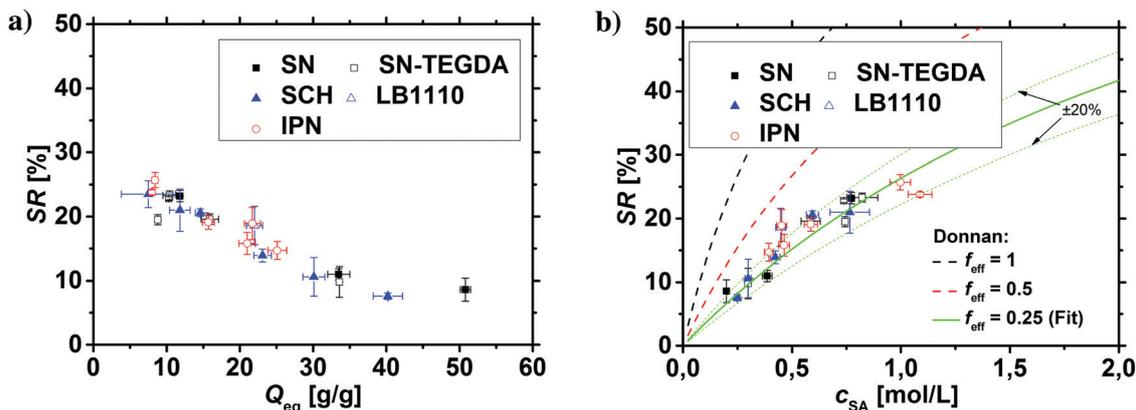
Fig. 11 (a) The salt rejection SR of the various hydrogel networks from this paper (see Table 1) is plotted as a function of the degree of swelling  $Q_{eq}$ . (b) SR as a function of the sodium acrylate concentration  $c_{SA}$ . A higher  $c_{SA}$  leads to a higher charge density and thus, to a better salt rejection. The experimental data are compared with calculations from the mean-field Donnan theory using different effective charge fractions ( $f_{eff}$ ).
