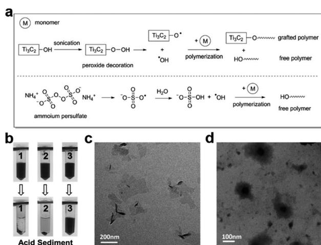
Fig. 4 (a) The proposed mechanism of polymerization initiated by p- $\text{Ti}_3\text{C}_2\text{T}_x$  or ammonium persulfate. (b) Acid stability of three p- $\text{Ti}_3\text{C}_2\text{T}_x$ -containing dispersions. Sample 1: pristine p- $\text{Ti}_3\text{C}_2\text{T}_x$ ; Sample 2: physical mixture of PNIPAM and p- $\text{Ti}_3\text{C}_2\text{T}_x$ ; Sample 3: PNIPAM-based NC polymer. The TEM image of p- $\text{Ti}_3\text{C}_2\text{T}_x$  (c) and the PNIPAM-based NC polymer (d).
