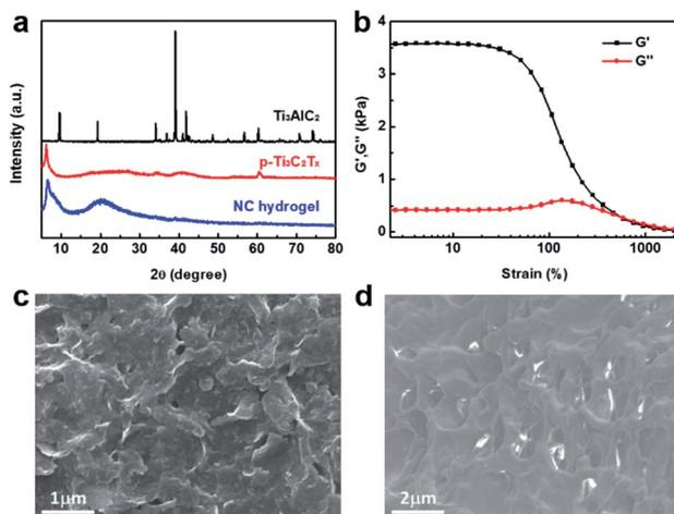
Fig. 1 (a) XRD patterns of  $\text{Ti}_3\text{AlC}_2$ ,  $p\text{-Ti}_3\text{C}_2\text{T}_x$  and PNIPAM-based NC hydrogels. (b) The storage and loss moduli of PNIPAM-based NC hydrogels obtained by continuous strain sweep at  $25^\circ\text{C}$ . SEM images of the  $p\text{-Ti}_3\text{C}_2\text{T}_x$  (c) and the PNIPAM-based NC hydrogels (d).
