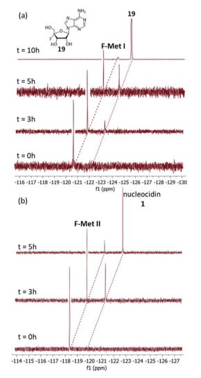
Fig. 6  $^{19}$ F{ $^1$ H}-NMR time course profiles of biotransformations of F-Mets I and II with  $\beta$ -glucosidase NucGS. (a) F-Met I is converted to 4′-fluoroadenosine 19. (b) F-Met II is converted to nucleocidin 1.
