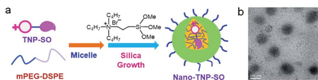
Scheme 2 (a) Schematic illustration of the generation of Nano-TNP-SO. (b) Characterization of Nano-TNP-SO by TEM. Scale bars: 100 nm.
