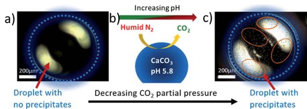
Fig. 5 (a) Dark field microscopy image of a calcium carbonate rich droplet in the *in situ* cell under 0.5 bar carbon dioxide partial pressure and high relative humidity  $90 \pm 5\%$ , (b) a schematic representation of the reaction in the cell and (c) dark field microscope image of calcium carbonate rich droplet while decreasing the carbon dioxide partial pressure to 0 bar shows (precipitates can be seen as dark spots in the droplet).
