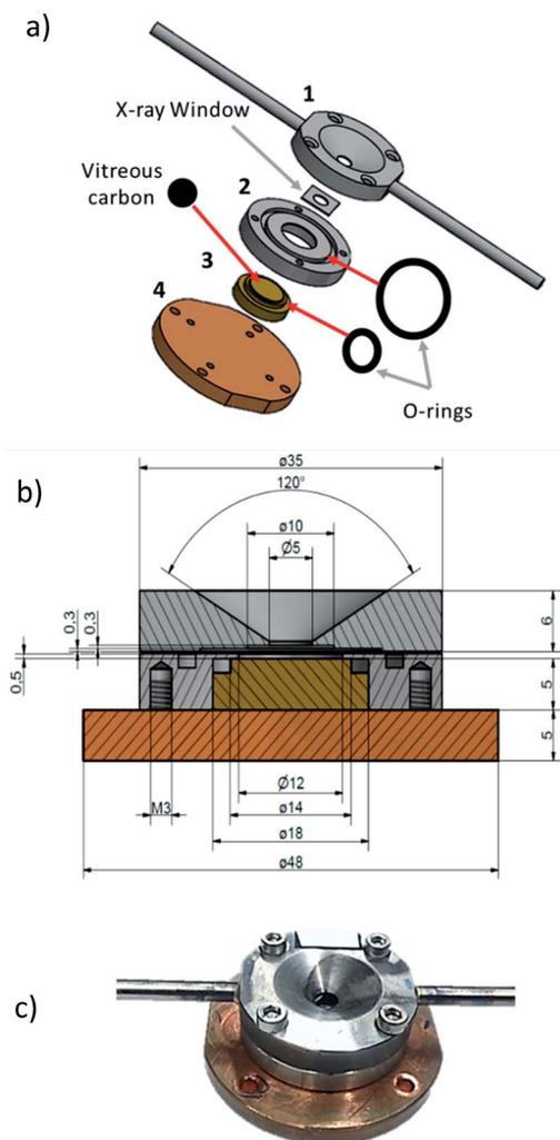
Fig. 1 (a) Schematic diagram of the individual cell parts of the *in situ* cell, (b) cross-section of the cell with dimensions in mm and (c) picture of the cell when closed and ready for mounting in the vacuum chamber.
