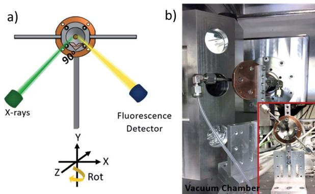
Fig. 2 (a) Schematic representation of the sample mounting geometry with respect to the incoming X-rays and the fluorescence detector and (b) picture of the *in situ* cell mounted in the vacuum chamber of the PHOENIX beamline at the Swiss Light Source (inset front view of the cell before mounting).
