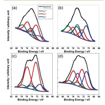
Fig. 6 XPS analysis of the Pt  $4f_{7/2}$  and  $4f_{5/2}$ : (a) Pt/TiO<sub>2</sub> as made, (b) Pt/TiO<sub>2</sub> after EF, (c) Pt/CeO<sub>2</sub> as made, and (d) Pt/CeO<sub>2</sub> after EF.
