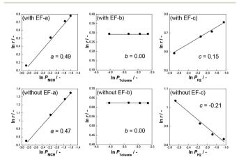
Fig. 2 Partial pressure dependences of (a) methylcyclohexane, (b) toluene, and (c) hydrogen over  $Pt/TiO_2$  for MCH dehydrogenation. Reaction temperature 423 K (with EF), 498 K (without EF), and input current 3 mA.
