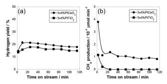
Fig. 4 Results of catalytic activity tests in the electric field over  $Pt/TiO_2$  and  $Pt/CeO_2$  at 423 K: (a) hydrogen yield and (b)  $CH_4$  by-production rate.
