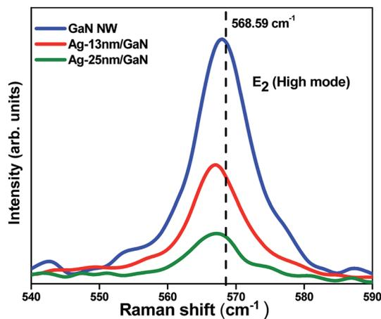
Fig. 4 Raman spectra showing  $E_2$  (high) mode of GaN nanowall network, Ag-13 nm/GaN and Ag-25 nm/GaN samples.
