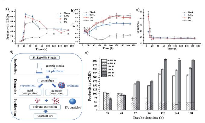
Fig. 2 Biosurfactant production with FA-based platform: (a) productivity of growth medium; (b) pH of growth medium; (c) ST of growth medium, (d) flow chart of the biosurfactant production process and (e) biosurfactant production in culture broth (0.5% L, 1% L, 2% L) and in FA particles (0.5% D, 1% D, 2% D).
