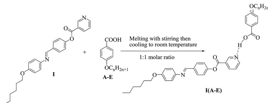
Scheme 2 Preparation of 1 : 1 supramolecular hydrogen-bonded complexes (I(A-E)).
