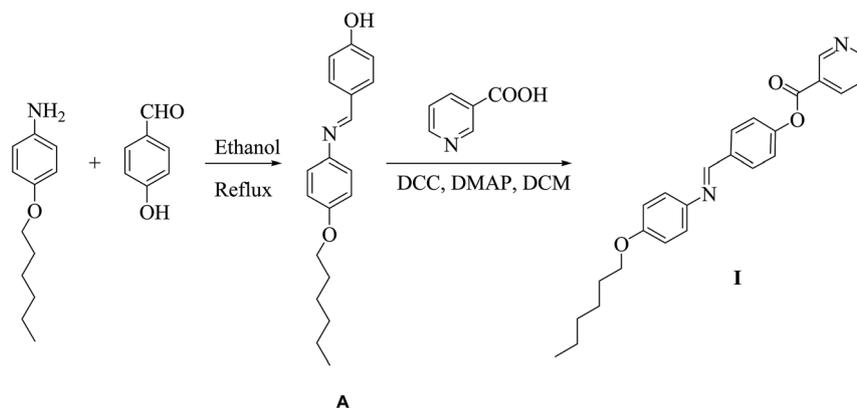
Scheme 1 Preparation of 4-(4-(hexyloxyphenylimino) methyl)phenyl nicotinate (I).
