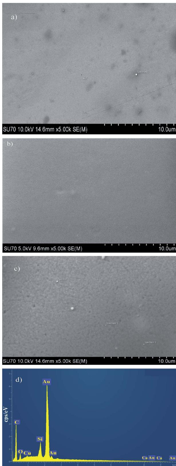
Fig. 8 SEM/EDX images of coated gold sensors (a) KL (b) PS (c) KL-PS (d) EDX of KL-PS image after Cu(II) adsorption. The sharp Au signal comes from the gold sensor.
