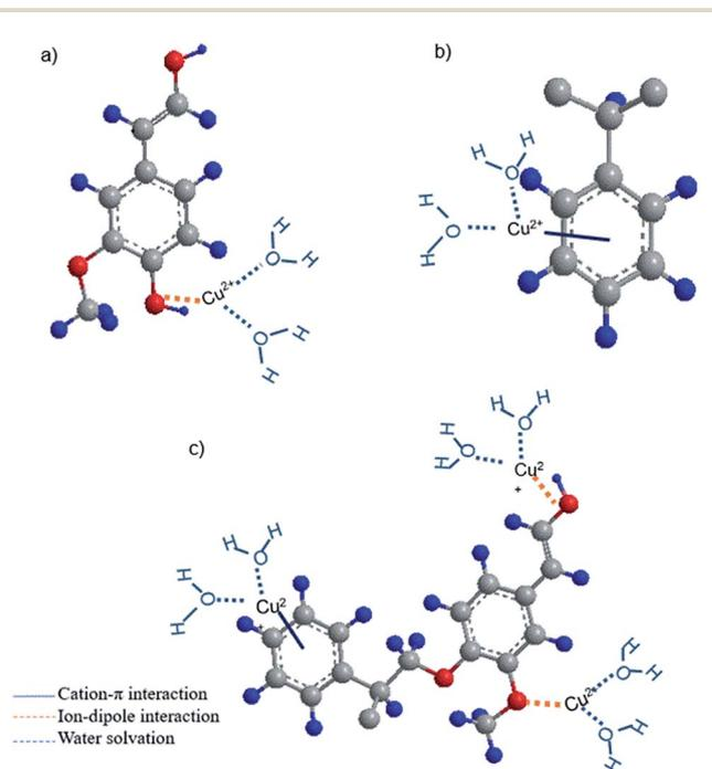
Fig. 7 The possible interactions of copper ions and (a) KL (b) PS (c) KL–PS substrates. Grey, red and blue balls represent carbon, oxygen and hydrogen atoms, respectively. For simplicity, only one unit of lignin or polystyrene is presented.
