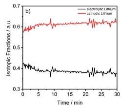
Fig. 5 Lithium abundances from Fig. 2(a) and (b) transformed into the electrolytic and cathodic fractions for the different components and aging conditions.
