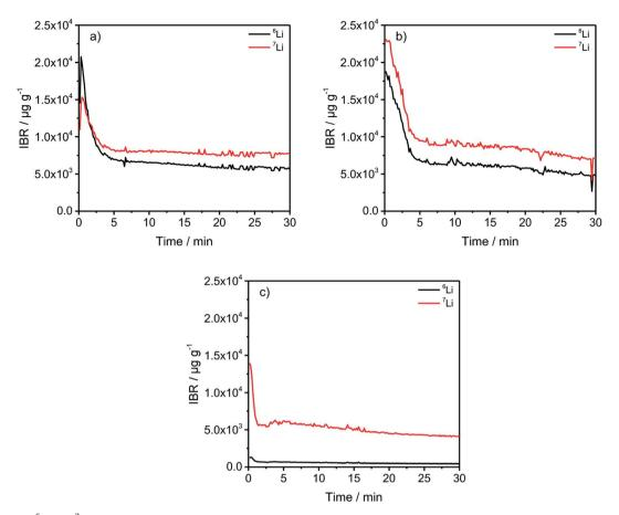
Fig. 3 IBRs for the  $^6$ Li and  $^7$ Li signals of differently aged, discharged anodes. (a) one formation step with C/5; (b) three formation steps with C/5 plus ten additional cycles with C/1; (c) one formation step with C/5 and the reference electrolyte cycled using the same procedure as the enriched cells for one formation step.
