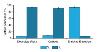
Fig. 1 Determined isotope abundances for the different pristine materials including the two used electrolytes, a cathode, (N = 3).
