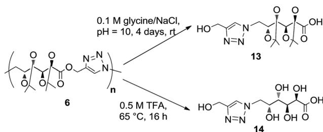
Scheme 4 Products of hydrolytic degradation of poly(ester-triazole) 6.
