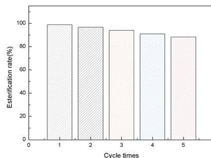
Fig. 10 Reusability of [TEAPS]<sub>5</sub>PW<sub>10</sub>V<sub>2</sub>O<sub>40</sub> catalyst on the esterification reaction.
