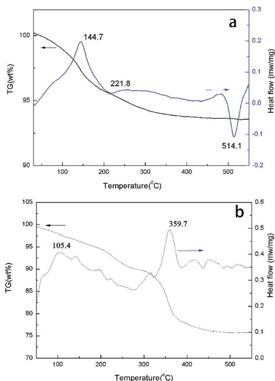
Fig. 6 TG-DSC plots of H<sub>5</sub>PW<sub>10</sub>V<sub>2</sub>O<sub>40</sub> (a) and [TEAPS]<sub>5</sub>PW<sub>10</sub>V<sub>2</sub>O<sub>40</sub> (b).
