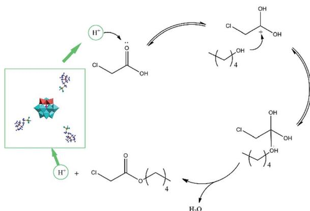
Fig. 9 Esterification reaction mechanism of chloroacetic acid using [TEAPS]<sub>5</sub>PW<sub>10</sub>V<sub>2</sub>O<sub>40</sub> catalyst.
