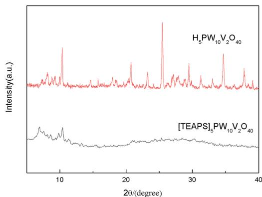
Fig. 5 XRD patterns of H<sub>5</sub>PW<sub>10</sub>V<sub>2</sub>O<sub>40</sub> and [TEAPS]<sub>5</sub>PW<sub>10</sub>V<sub>2</sub>O<sub>40</sub>.
