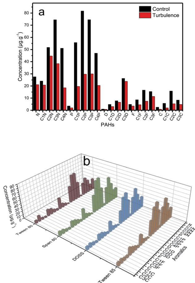
Fig. 9 Distributions of PAHs in the sediment 96 hours prepared with turbulence in 120 rpm (a) and four dispersant (b), respectively, at a fixed DOR of 1 : 20.
