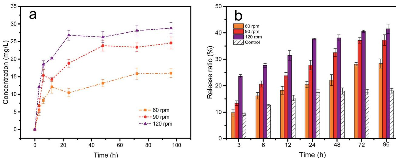
Fig. 5 Effect of turbulence on petroleum hydrocarbon concentration (a) and release ratio (b) at the 60, 90, 120 rpm in 18.21 mg g<sup>-1</sup> contamination levels.
