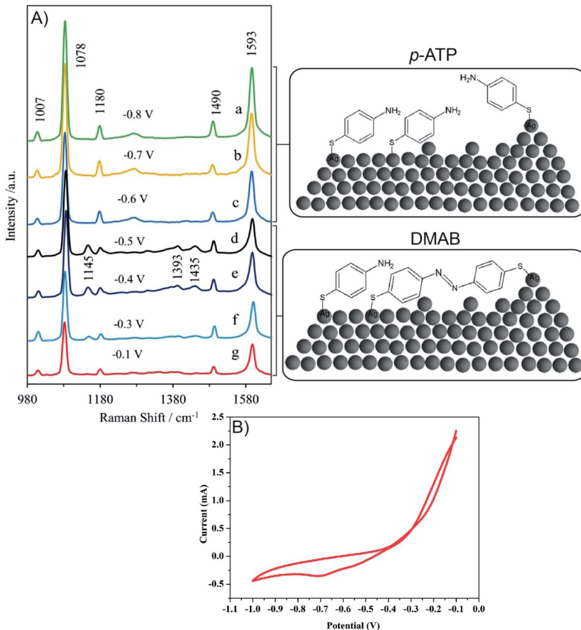
Fig. 10 (A) Potential dependent SERS spectra of *p*-ATP adsorbed onto Ag/PV SERS surface from  $10^{-6}$  M solution of *p*-ATP in 0.1 M NaClO<sub>4</sub>, "in situ" measurements. (B) Cyclic voltammogram recorded during spectroelectrochemical measurements.
