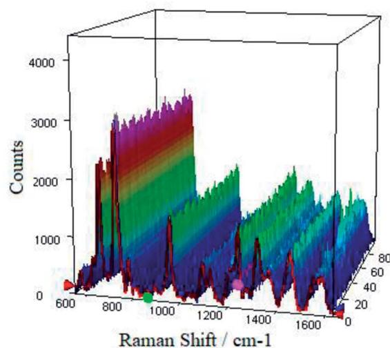
Fig. 9 The representative SERS spectra of (A and B)  $p$ -ATP of concentration  $10^{-6}$  M, (C) *E. coli*, and (D) *B. subtilis* recorded from 40 different spots on the SERS surface (type 1m) using mapping mode.
