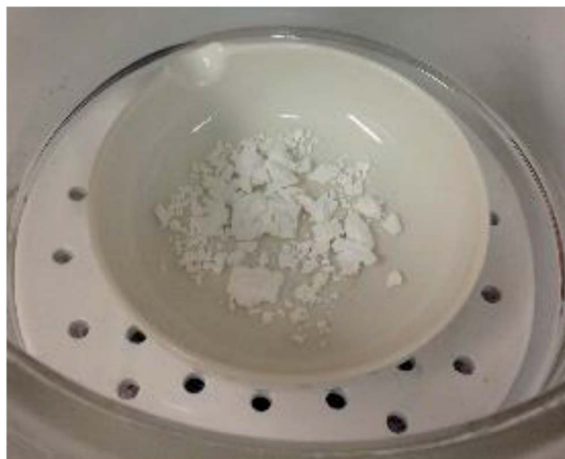
Fig. 7 Mixed yttrium/europium oxide obtained via the recovery process described in present work.
