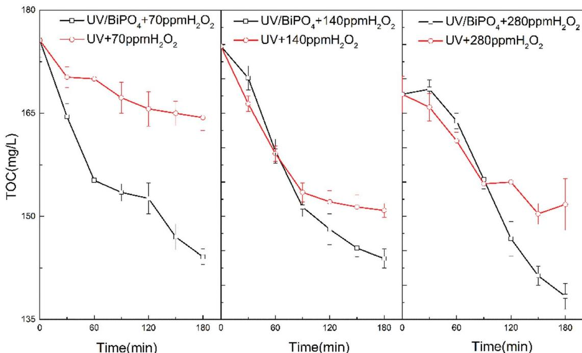
Fig. 6 Effect of different H<sub>2</sub>O<sub>2</sub> residues of the H<sub>2</sub>O<sub>2</sub>/O<sub>3</sub> pre-treatment on the TOC removal: parameters carried out according to Run 2 with 74.47 mg L<sup>-1</sup> H<sub>2</sub>O<sub>2</sub> residues, Run 3 with 138.10 mg L<sup>-1</sup> H<sub>2</sub>O<sub>2</sub> residues and Run 3 with 239.53 mg L<sup>-1</sup> H<sub>2</sub>O<sub>2</sub> residues.
