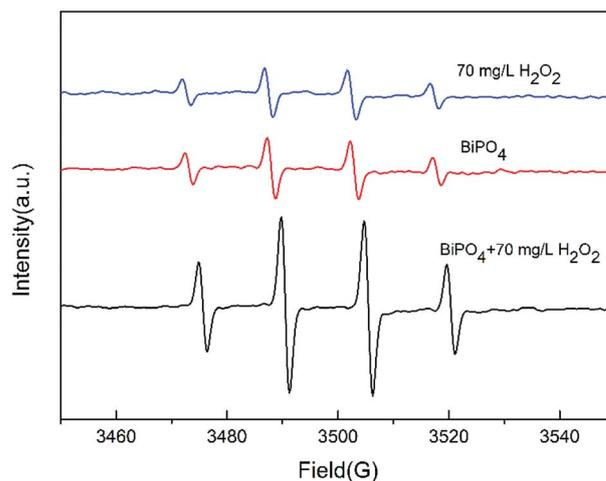
Fig. 5 DMPO spin-trapping ESR spectra under UV irradiation for 2 min at room temperature water in the presence of  $\text{BiPO}_4$ ,  $\text{H}_2\text{O}_2$  or both  $\text{BiPO}_4$  and  $\text{H}_2\text{O}_2$ .
