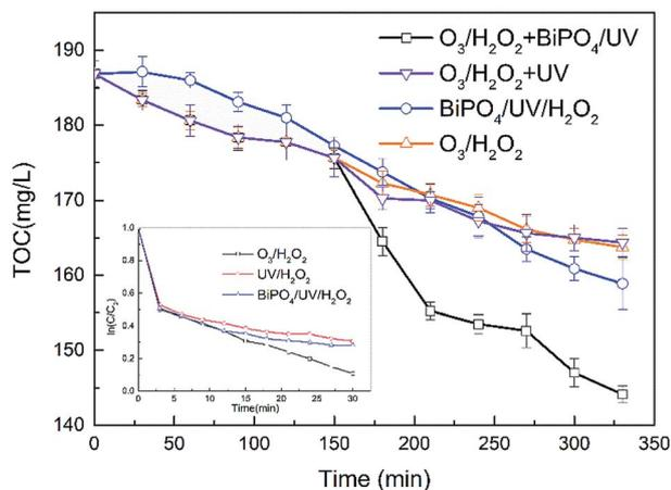
Fig. 3 Comparison of mineralization efficiencies among O<sub>3</sub>/H<sub>2</sub>O<sub>2</sub> + BiPO<sub>4</sub>/UV synergy technique, O<sub>3</sub>/H<sub>2</sub>O<sub>2</sub> + UV, O<sub>3</sub>/H<sub>2</sub>O<sub>2</sub> and BiPO<sub>4</sub>/UV/H<sub>2</sub>O<sub>2</sub> processes and the degradation efficiencies among O<sub>3</sub>/H<sub>2</sub>O<sub>2</sub>, UV/H<sub>2</sub>O<sub>2</sub> and BiPO<sub>4</sub>/UV/H<sub>2</sub>O<sub>2</sub>.
