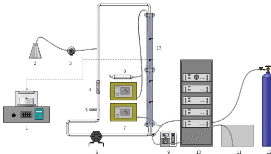
Fig. 1 Experiment reactor. (1): Photoreactor instrument; (2): agents can for  $\text{H}_2\text{O}_2$ ; (3): agents pump; (4): flowmeter; (5): pH-meter; (6): circulating pump; (7): ozone meter; (8): ozone destructor; (9): peristaltic pump; (10): ozonator; (11): wastewater tank; (12): oxygen bottle; (13): reaction tower.
