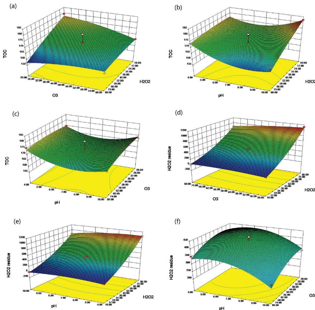
Fig. 2 Interaction effects of different parameters on TOC (a–c) and H<sub>2</sub>O<sub>2</sub> residues (d–f) using 3D response surface and 2D contours: (a) O<sub>3</sub> concentration and initial H<sub>2</sub>O<sub>2</sub> dosage, (b) pH and H<sub>2</sub>O<sub>2</sub> dosage, (c) pH and O<sub>3</sub> concentration, (d) O<sub>3</sub> concentration and H<sub>2</sub>O<sub>2</sub> dosage, (e) pH and H<sub>2</sub>O<sub>2</sub> dosage, (f) pH and O<sub>3</sub> concentration.
