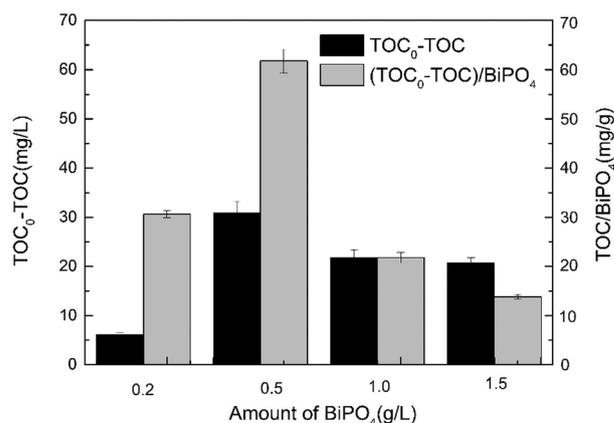
Fig. 8 TOC removal amount and  $(\text{TOC}_0 - \text{TOC})/\text{BiPO}_4$  ratio in the post-treatment process. The TOC amount after pre-treatment was 174.5  $\text{mg L}^{-1}$ ,  $\text{H}_2\text{O}_2$  residue was 71.45  $\text{mg L}^{-1}$ , and UV intensity was 4.73  $\text{mW cm}^{-2}$ .
