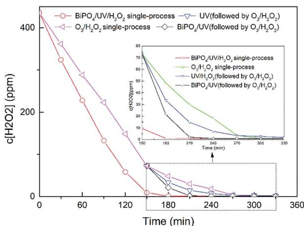
Fig. 4 Comparison of  $\text{H}_2\text{O}_2$  utilization in different processes. The concentration of thiourea was  $1.2 \text{ g L}^{-1}$ , the concentration of ammonia nitrogen was  $140 \text{ mg L}^{-1}$ , the initial concentration of  $\text{H}_2\text{O}_2$  was  $435 \text{ mg L}^{-1}$ ,  $\text{O}_3$  concentration was  $55.71 \text{ mg L}^{-1}$ , UV intensity was  $4.73 \text{ mW cm}^{-2}$ , and the  $\text{BiPO}_4$  loading was  $0.5 \text{ g L}^{-1}$ .
