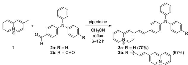
Scheme 1 Synthesis of styrylquinolizinium derivatives **3a** and **3b**.
