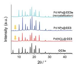
Fig. 4 PXRD patterns for CC3 (black), desolvated 0.5 wt%  $Pd(NO_3)_2$ @CC3 (red), 0.5 wt% Pd NPs@CC3 after  $H_2$  reduction at 200 °C for 1 hour (blue), and recrystallization of 0.5 wt% Pd NPs@CC3 in DCM to form pure CC3α phase (cyan). Yellow arrows denote additional reflection at 7.6°.
