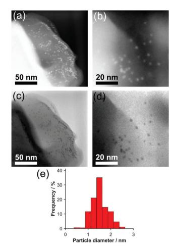
Fig. 3 (a and b) dark field and (c and d) bright field STEM images of 0.5 wt% Pd NPs@CC3. (e) Size histogram of Pd NP diameters.
