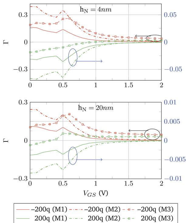
Fig. 9 Change in the transfer curve of the device when molecules are included in the simulations. The molecular charge is set to  $-200q$  (orange) and  $200q$  (blue) using the three interaction models. Models 1 and 2 depict a similar behaviour (quite symmetric with respect to the sign of  $Q_M$  and scaled down when  $h_M$  increases), while Model 3 exhibits a different behaviour.
