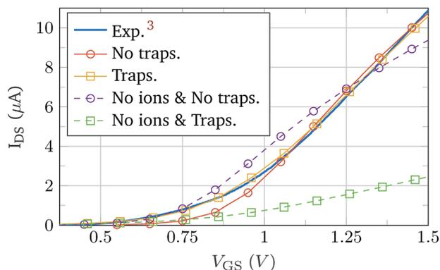
Fig. 5 Comparison between the data measured by Sarkar *et al.*<sup>3</sup> (solid blue) and the results of the BioFET simulations, with ions (solid) and without ions (dashed). Markers indicate whether interface traps are considered in the simulations (squares) or not (circles).
