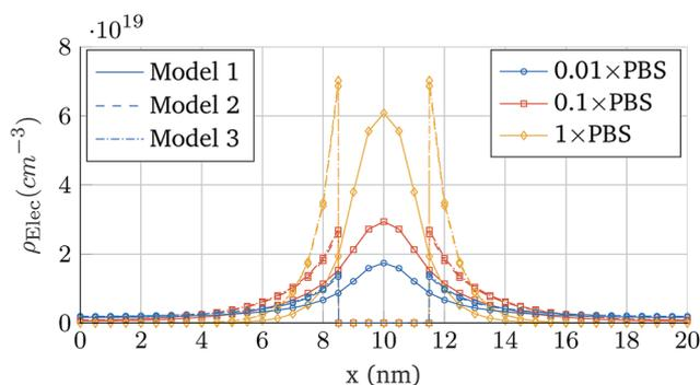
Fig. 7 Longitudinal charge density profiles at  $y = 6$  nm. The cases depicted correspond to the three interaction models when the PBS concentration is modified:  $0.01 \times$  PBS,  $0.1 \times$  PBS and  $1 \times$  PBS.
